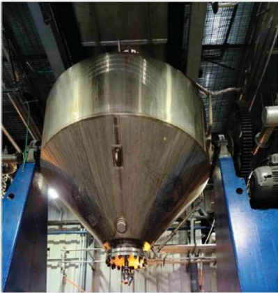
Figure 2. Optima Belle's rotary double cone jacketed dryer. (Credit: Optima Belle)
